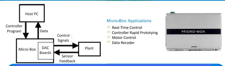
Real Time Control Systems: Micro-Box with MathWorks's xPC Target
